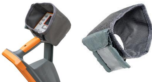
Fig. 8 Receiver with sun-protective cover
